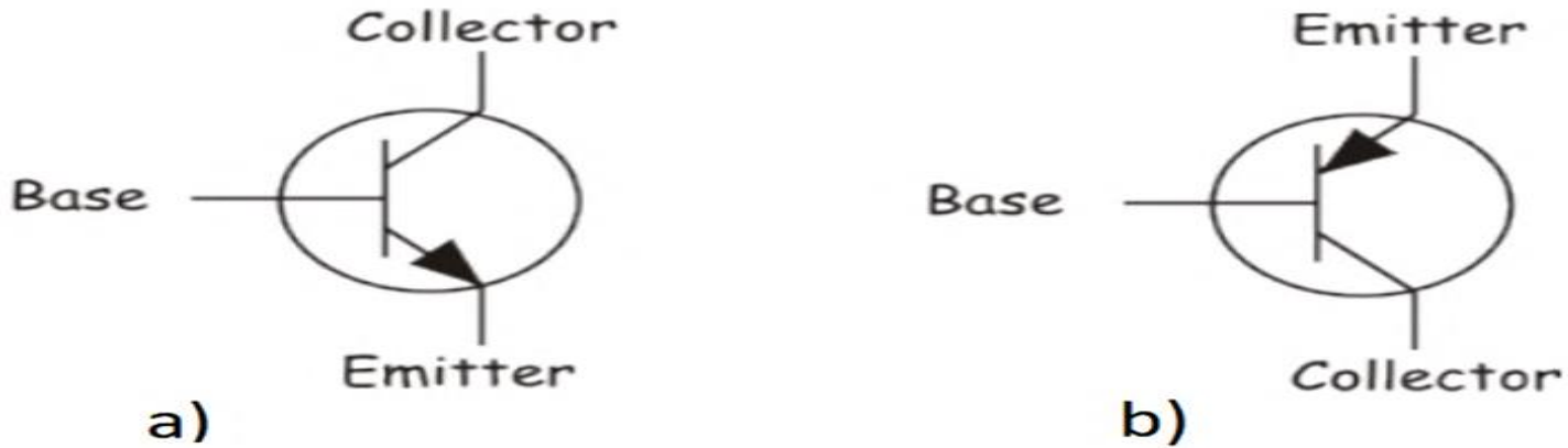
Figure: Schematic symbol for (a) NPN transistor & (b) PNP transistor.
